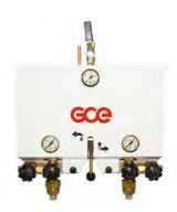
Manifold MM40 Semiauto is a semi-automatic manifold. It is working on principal different pressure between the operation and reserve regulator. By the manual lever, operator can decide which side will be the operational one and which will be the reserve one. When the operating side is empty, the manifold will without any action start to supply gas from the reserve side with the lower regulator pressure and fulfill the requests to supply without interrupting the flow.
