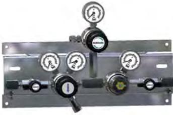
**Dual-stage, for inert, reactive, flammable and oxidizing gases and gas mixtures, purity max. 5.0, inlet pressure 230 bar / 3300 psi, preset downstream pressure 14 bar - 200 psi**
