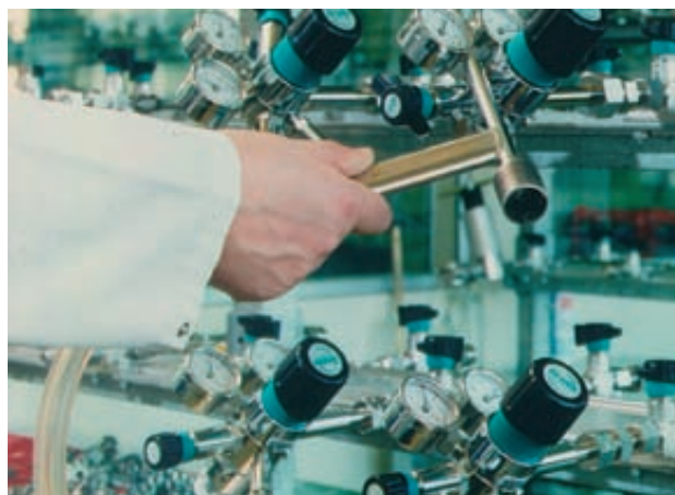
Helium leak testing
