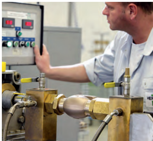
100 % tightness test of the valves at design pressure
